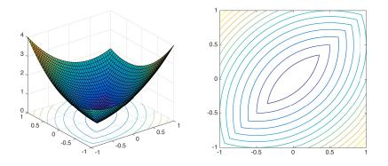
Figure 10.1: The non-differentiable function  $f(\mathbf{x}) := ||\mathbf{x}||^2 + |x_1 - x_2|$ . The global minimum is (0,0), but greedy coordinate descent cannot escape any point  $(x, x), |x| \le 1/2$ . Figure by Alp Yurtsever & Volkan Cevher, EPFL
